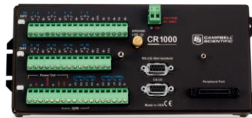
Figure 2: Campbell Scientific CR1000 Data Logger
